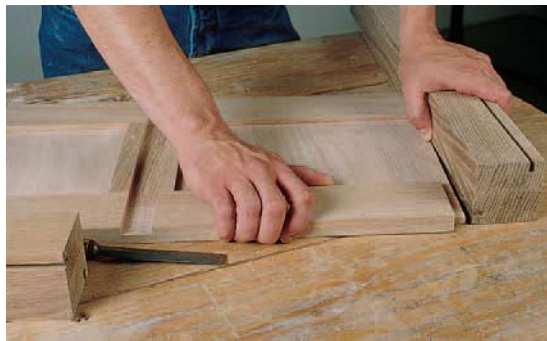
Figure 3: Before final assembly, test fit the joints between pre-made subassemblies, such as the back sub-assembly and the legs.
