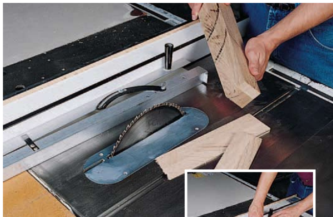
Figure 1: Tapering the outside faces of the legs adds an element of style to their blocky, rectangular shapes.
